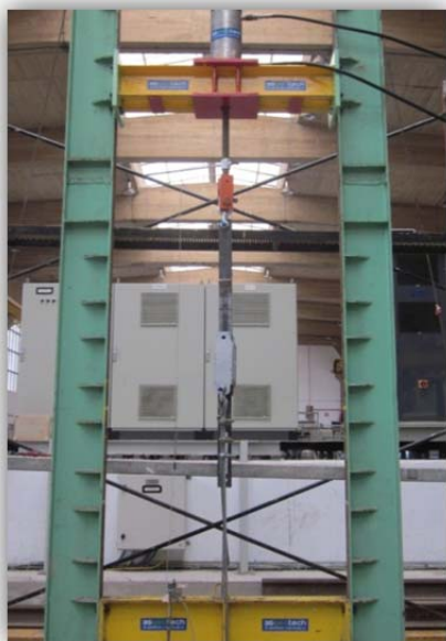
Certification tests of dissipaters type 3S-DPL in collaboration with Cantabria University
